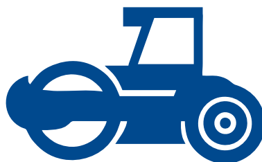
Large roller: Keep 3 feet away from wall face
