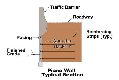
**Piano Wall™** is a combination precast traffic barrier and Mechanically Stabilized Earth (MSE) retaining wall. The lower portion of each unit serves as the precast concrete facing for the MSE wall and the upper section serves as an integral Jersey-type traffic barrier.
