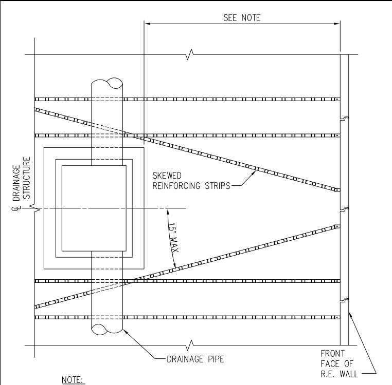
AN IDEAL DRAINAGE STRUCTURE SETBACK IS ONE SUFFICIENT TO PERMIT STRIPS TO BE SKEWED ≤ 15° TO CLEAR STRUCTURE
