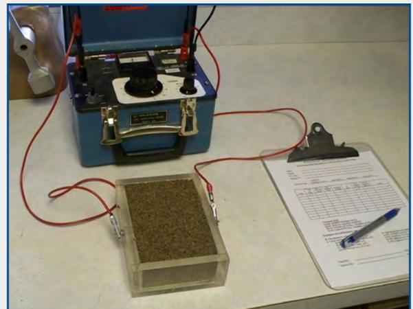
Figure 1 - Typical Resistivity Test Setup
