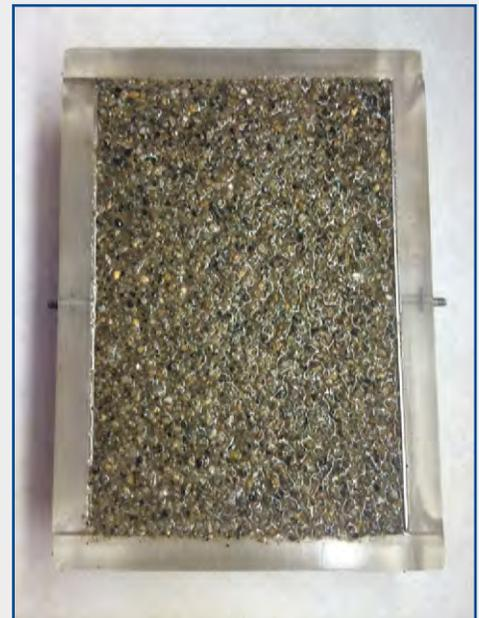
Figure 3 - Sheen on Soil Sample after Adding Water
