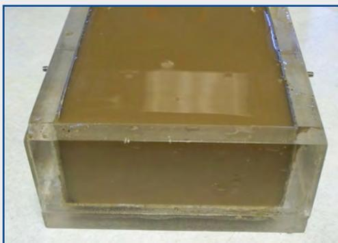
Figure 2 - Test Box with Slurry (no backfill solids, only water)
