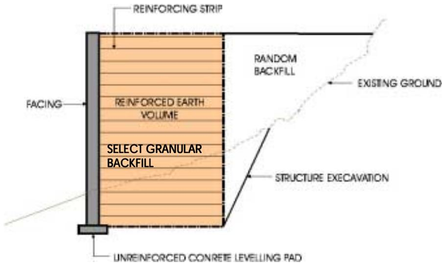
**FIGURE 2 - COMPONENTS OF AN MSE WALL**
