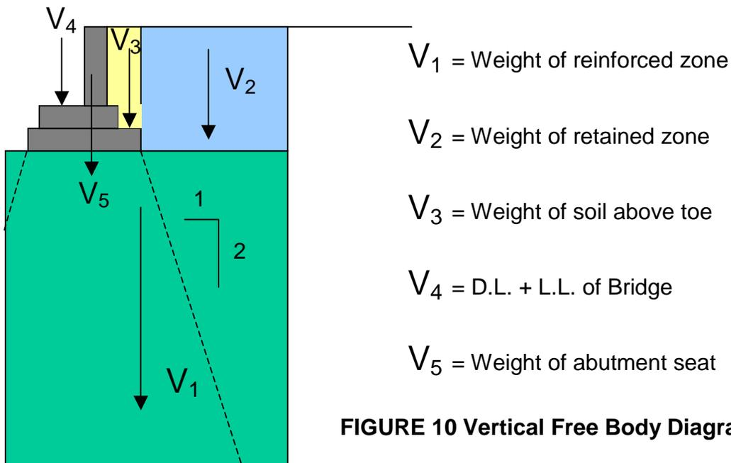
**FIGURE 10 Vertical Free Body Diagram**
